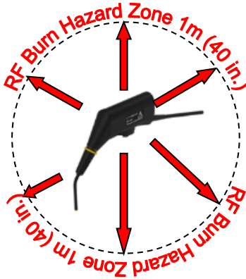
RF burn hazard zone around the probe head and tip cable
